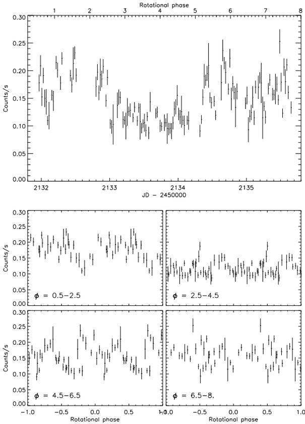
**Fig. 4.** *Top panel:* MECS quiescent light curve observed in August 2001 (all obvious peaks have been removed). *Bottom panels:* MECS folded light curve divided into four equal intervals lasting 2 rotational periods
