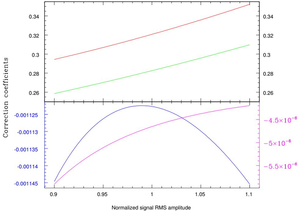
Figure 2: Polynomial coefficients of the correction function for 2 bit quantization. Horizontal scale is the signal RMS amplitude. Curves represent: red  $a'$ , blue  $b'$ , violet  $c'$ , green  $R/R_4$  for  $\rho = 1$
