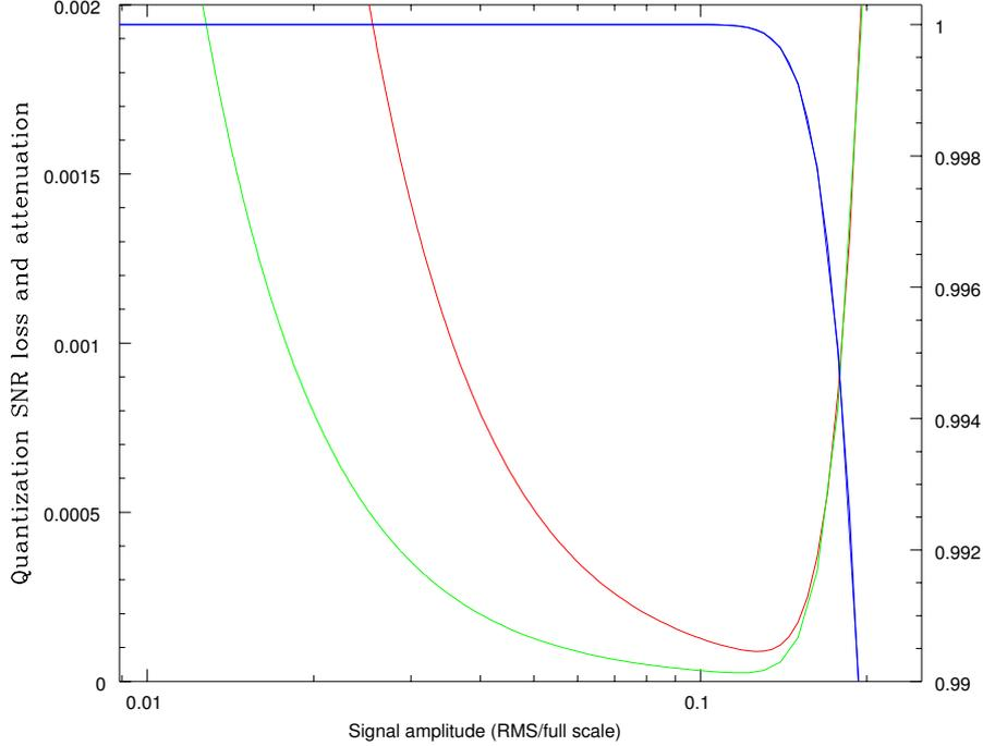
Figure 1: Gain (blue) and quantization loss for a 8 bit (red) and 9 bit (green) quantizers, as a function of the signal RMS level  $\sigma$  divided by the quantizer total range  $\alpha\sigma_e$
