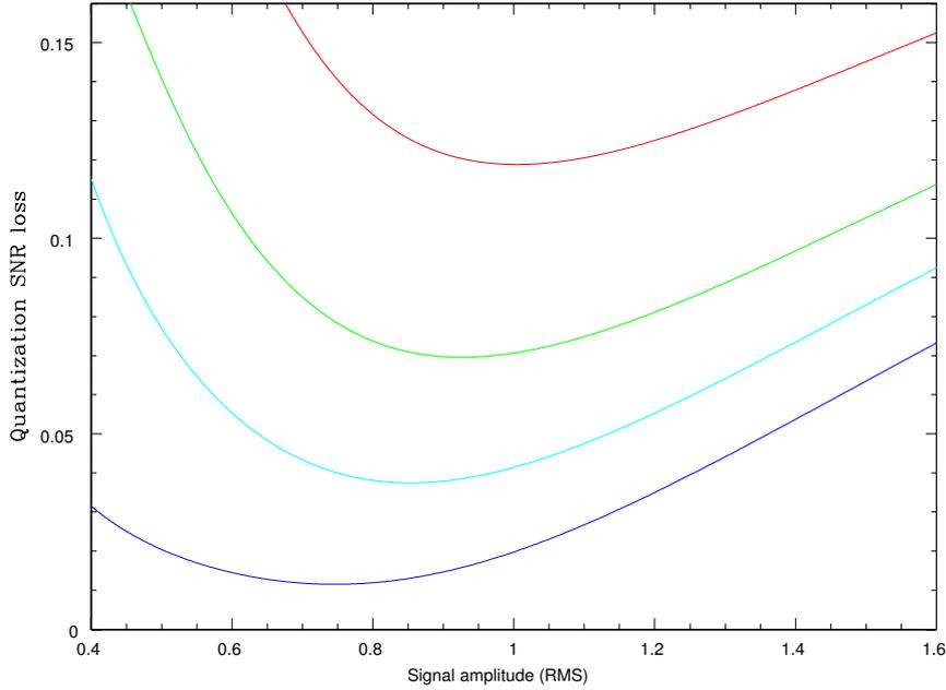
Figure 7: Quantization efficiency (left) for quantization schemes with: 2 bits, 4 level (red),  $2 \times 4$  bits (green), 3 bits (cyan) and 4 bits (blue). Horizontal scale corresponds to an amplitude from 0.4 to 1.6 times ( $-8$  to  $+4$  dB) the central threshold in the quantization scheme.
