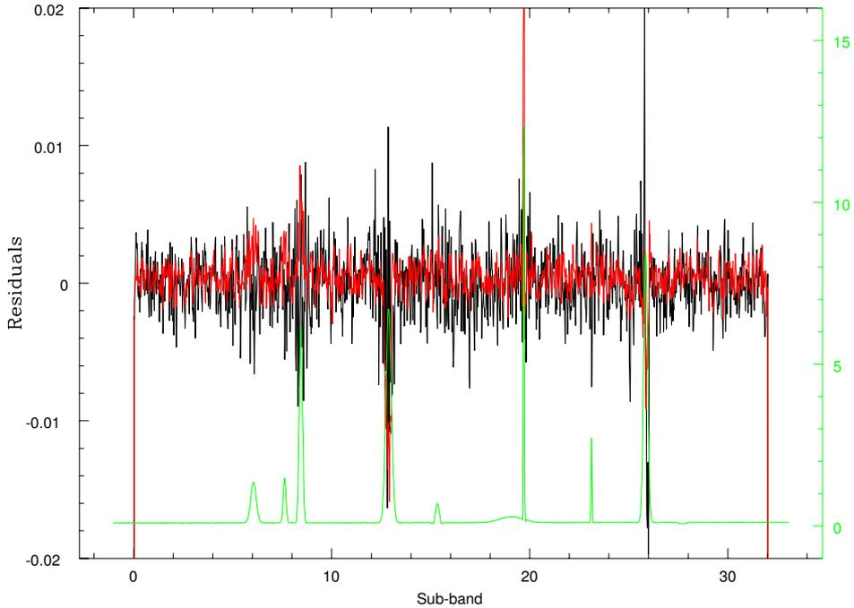
Figure 5: Residuals for the hybrid spectrum, both with (black) and without (red) final 2-bit requantization. Horizontal scale is in channels (0 to 31). Green line is the original cross spectrum, with scale on the right.
