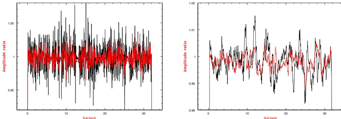
Figure 4: Ratio of hybrid cross spectrum to the original one. Horizontal scale is in channels (0 to 31). Left graph is for the full resolutions (64 channels/sub-channel), right is smoothed to 4 channels/sub-channel. Red graphs refers to signal processed by the filterbank but not quantized to 2 bit
