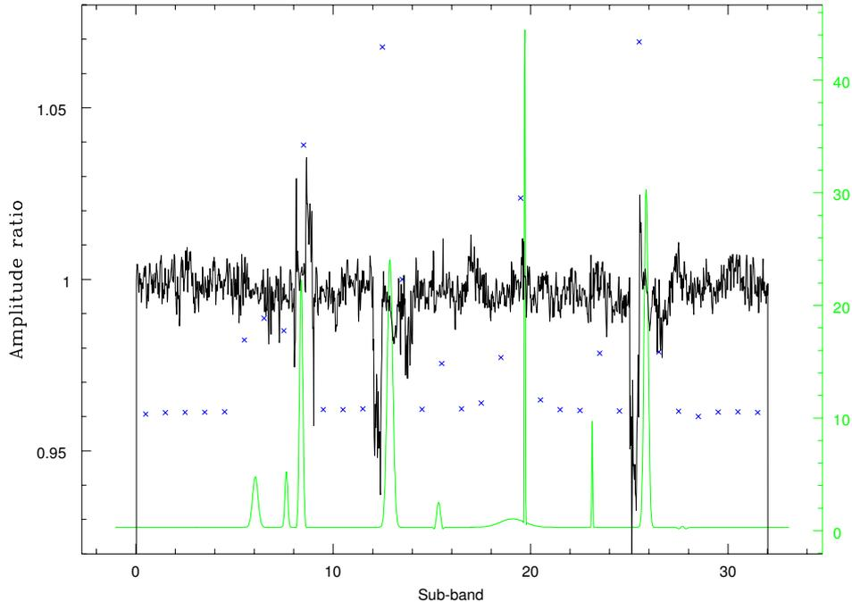
Figure 6: Ratio of hybrid cross spectrum to the original one. Horizontal scale is in channels (0 to 31). Green line is the original cross spectrum, with scale on the right. Blue crosses indicate RMS power in individual sub-channels, in arbitrary units (right scale).
