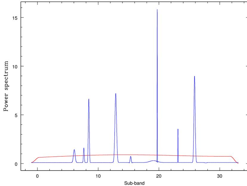
Figure 3: Test signal spectrum. Red is the uncorrelated part, and blue is the correlated one. Each spectral feature in the correlated part has a different phase. The correlated continuum level is 0.1. The spectrum is normalized to unity average spectral density. Horizontal scale is in channels (0 to 31).
