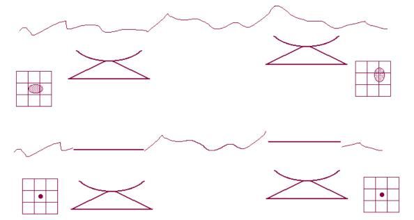
At the single telescope level, **active** and **adaptive** optics aim at generation of a focal plane image close to the diffraction limit
