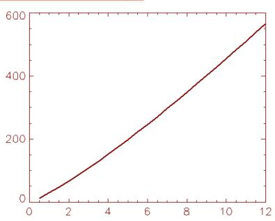
Coherence length [m] vs. wavelength [ $\mu m$ ]
